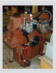
Vertical offset unit with extended shaft.
